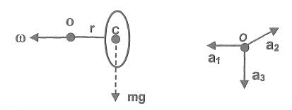
The gyroscope is released with an angular velocity  $\omega$  about its axis of symmetry  $a_1$  but with zero velocity of this axis.
