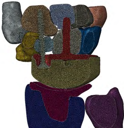
Caption: Finite element model of the implanted wrist
