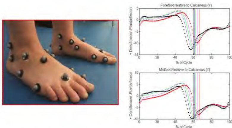
Figure 1: a) Picture of multisegment marker system, b) Example of changes in multisegment angles as a function of speed (black = very fast; red = very slow)
