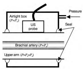
Figure 1: Schematic diagram of the transmural pressure manipulation method.
