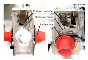
Figure 2: The airtight chamber with a US probe.
