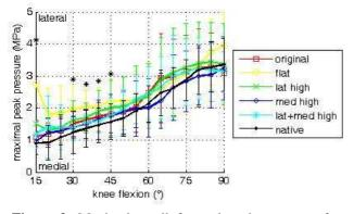
**Figure 2:** Maximal patellofemoral peak pressure after TKA with the 5 different designs compared to the native knee.
