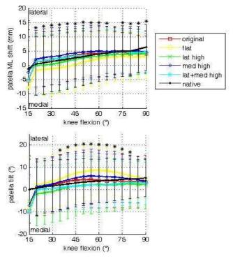
**Figure 1:** Mediolateral shift and tilt of the patella with respect to the femur after TKA with the 5 different designs – original Genesis II, completely flat, laterally elevated (lat high), medially elevated (med high) as well as laterally and medially elevated (lat+med high) – compared to the native knee.
