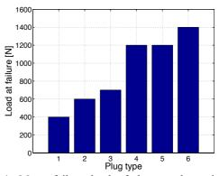
Figure 1: Mean failure load of the tested specimen (1unlocked, 2-Synthes® End Caps, 3-Hofer® Plug 3mm, 4-Hofer® Plug 3.5mm, 5-Hofer® Fix Plug, 6-Hofer® Twin Plug)
