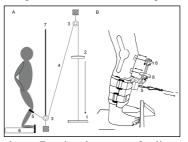
Figure 1: Schematic drawing of the experimental setup. A: Experimental setup, B: Measurement system | 1: stopper, 2: falling weight, 3: pulley, 4: steel rope, 5: force transducer, 6: force potentiometer. Arrows
