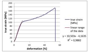
Figure 1. Tensile test of the hair
