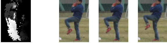
Figure 3: MHI (left) and the snapshots of the corresponding image sequence (right). The motion is raising the left leg.
