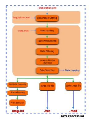
Figure 2: Flowchart of steps in the Data Processing part.
