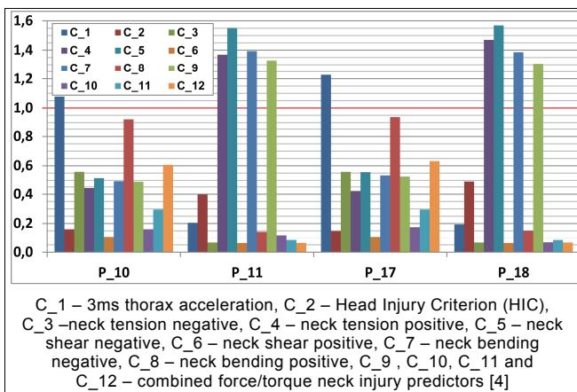
**Figure 2:** Values of the 12 biomechanical injury indexes for the seat fixed on joints at points P\_10, P\_11, P\_17 and P\_18 relative to the individual values for the stiffly fixed seat.
