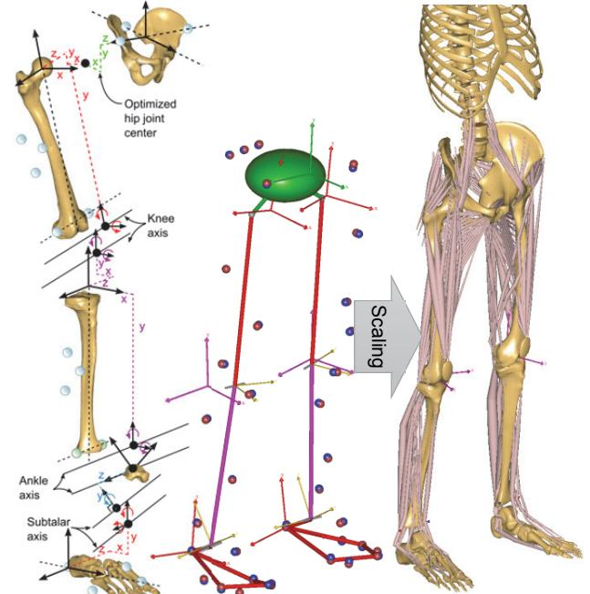
**Figure 2:** The patient-specific kinematic stick-figure model specifies the scaling/transformation of the musculoskeletal template geometry.
