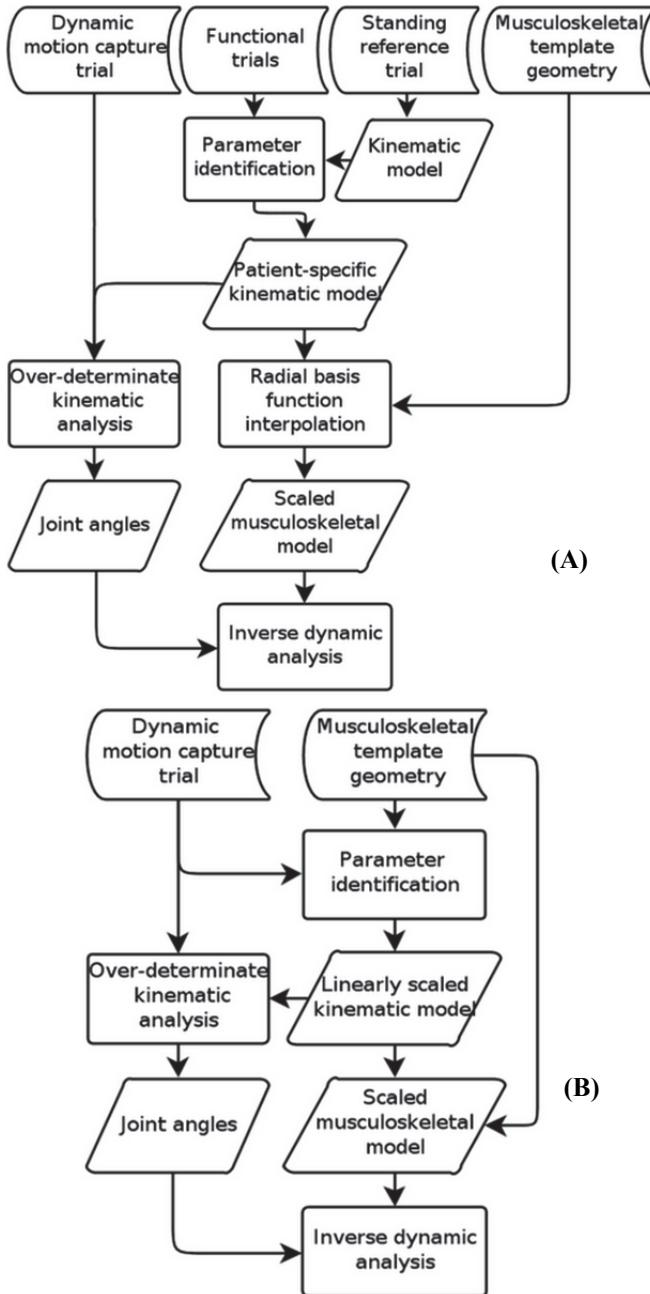
**Figure 1:** Schematic overview of the models. A) The *Kinematically scaled model* uses a standing reference and functional trials to obtain a patient-specific kinematic model. B) The *Linearly scaled model* relies on the dynamic trial only to linearly scale the model.
