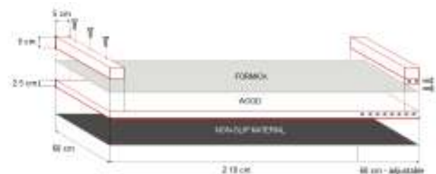
Figure 1: Slide board ergometer structure.
