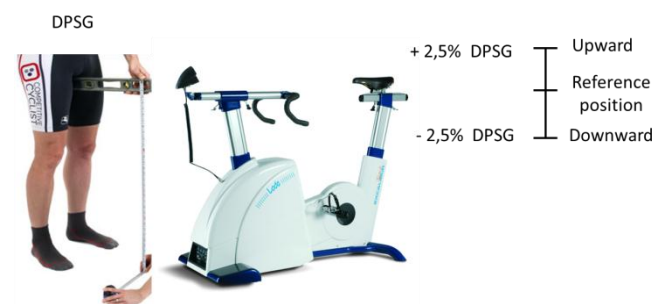
Figure 1. Saddle height measured from the distance from the pubic symphysis to the ground and the three positions during the Wingate tests: upward (+2.5% DPSG), reference position, and downward (-2.5% DPSG).
