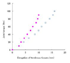
**Figure 1:** Typical examples of relation between joint torque and lengthening in tendinous tissues. (Open square: data from a subject in HPG, Filled square: data from a subject in NPG)
