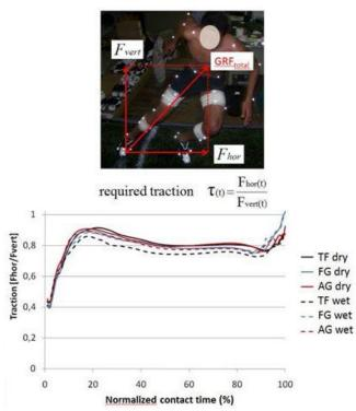
Figure 1: Temporal evolution of the required traction, calculated as ratio of the horizontal/vertical component of the ground reaction force [3], executed during the  $180^{\circ}$  turn by the outward foot; conditions: 3 shoe types (Turf Field, Artificial Grass, Firm Ground) x Wet and Dry AT. Average curves for 11 subjects.
