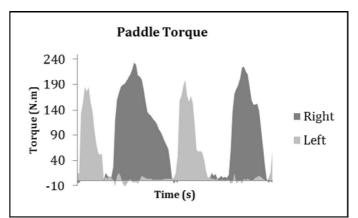
**Figure 1**: Four consecutive strokes showing the magnitude of the torque measured by the strain gauges on the instrumented paddle. The shaded area per stroke represents a summary variable for the amount of force applied by the paddler.
