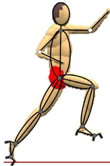
Figure 2: Thirteen-segment simulation model with wobbling masses within the shank, thigh, and trunk segments, torque drivers at the ball, ankle, knee, hip, and shoulder joints (grey circles), angle drivers at the elbow joints (white circles), and spring-dampers at three points on each foot.
