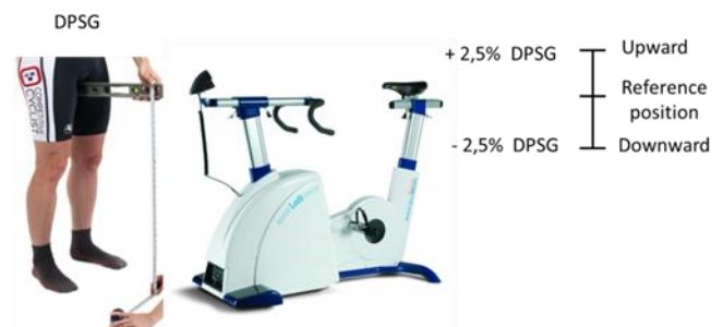
Figure 1. Saddle height calculated from the distance from the pubic symphysis to the ground and the three positions adopted during the Wingate tests: upward (+2.5% DPSG), reference position, and downward (-2.5% DPSG).
