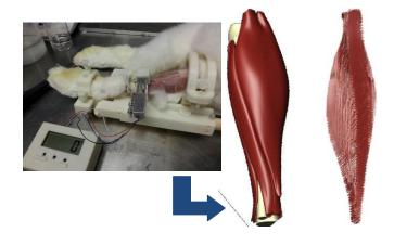
**Figure 1**: (Left) 3D printed MRI rabbit rig with force tranducer; (Middle) rabbit finite element model; and (Right) muscle fibers from DTI.
