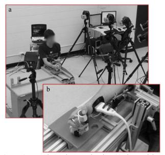
**Figure 1:** Experimental setup showing (a) the participant with the forearm immobilized in the apparatus, and (b) the custom handgrip used to perform long finger movements.
