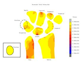
Figure 1: Minimum principal strains results for the minimum grip loading.
