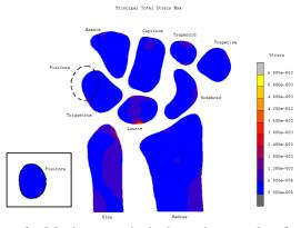
Figure 4: Maximum principal strains results for the maximum grip loading.
