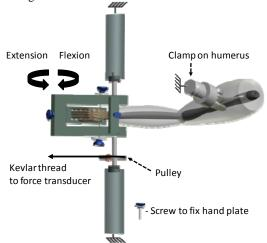
Figure 1: Schematic drawing of experimental setup. See [1] for a detailed description.
