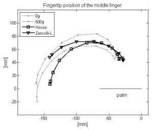
**Figure 1**: Fingertip position of the middle finger with different activation of the intrinsics (grey) and with two reconstruction procedures of the intrinsics (black).
