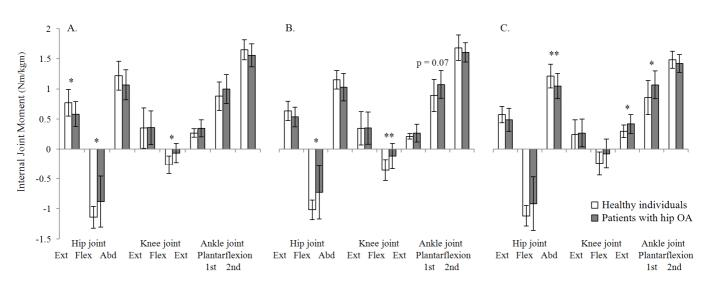
Figure 2: Group differences in internal joint moment during straight walk (A), step turn (B), and crossover turn (C). Positive values correspond to moment of hip extension and abduction, knee extension, and ankle plantarflexion. \*  $p \le 0.05$ , \*\*  $p \le 0.01$
