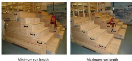
**Figure 1.** Custom-built staircases, highlighting the minimum (left) and maximum (right) run lengths used for testing. Note. A handrail (not shown in the picture) was present for all testing. However, subjects were instructed to ascend/descend without the handrail.
