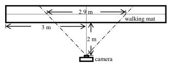
Figure 1: Overhead view of hardware setup.
