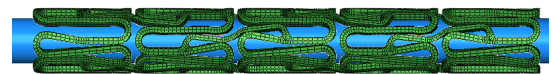
Figure 2: Hexahedral mesh of the Coroflex™ stent with a rigid cylinder inside used for the radial expansion
