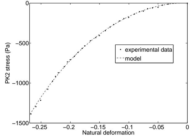
Figure 1: PK2 stress vs natural strain for the unconfined compression experiment (strain rate =  $0.64 \cdot 10^{-2} s^{-1}$ ). The experimental data comes from [3]
