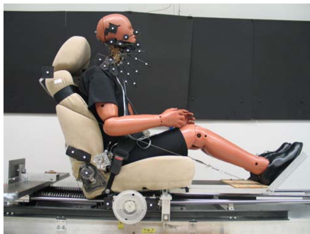
Figure 1. Photograph of the Human Model of the Neck (HUMON) and rear impact apparatus.
