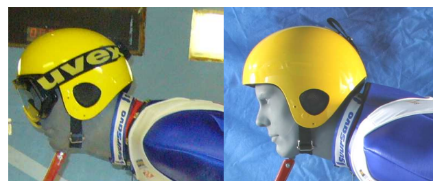
Figure 3: The effects of neckline diameter and modifications were tested. The shape of the neckline (right) was emphasized by inserting a thin steel wire to the seam of the suit.
