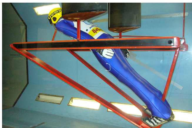
Figure 1: A full-scale doll model with the frame suspended from the wind tunnel balance.
