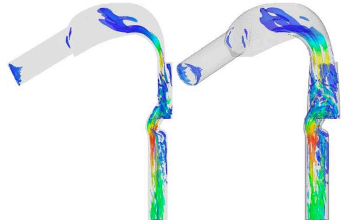
Figure 2: Iso-surface plot of  $Q$ -value ( $2^{\text{nd}}$  invariant of the velocity gradient tensor), by velocity magnitude. *Left* sagittal view. *Right* posterolateral ( $45^{\circ}$  oblique) view.
