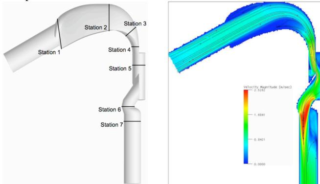
Figure 1: ETA geometry. *Left* Measurement stations. *Right* LBM velocity magnitude contours, sagittal plane.
