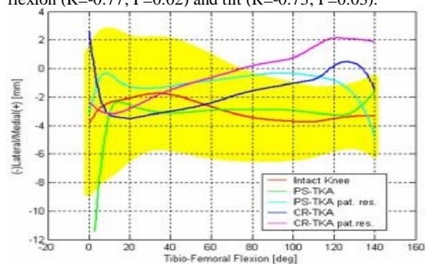
**Figure 1:** PFJ translation along femoral medio-lateral axis in the intact knee and after different TKA options.
