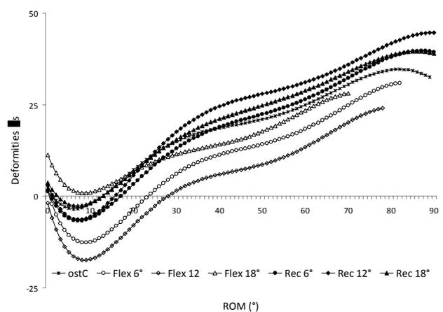
Figure 2: Variation of bone deformity for antero-medial strain gage during different conditions of bone correction.
