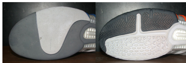
Figure 1: Photographs of the smooth shoe (left) and the cleated shoe (right) soles.
