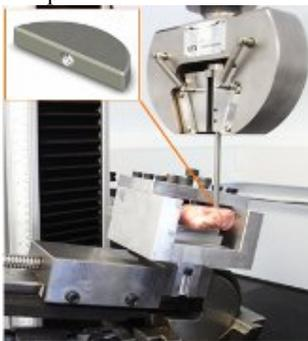
**Figure 1:** Implant geometry and push-out test set-up
