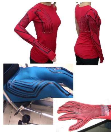
Figure 1: Sensorized Prototypes for monitoring the upper limb, the lower limb and the hand.
