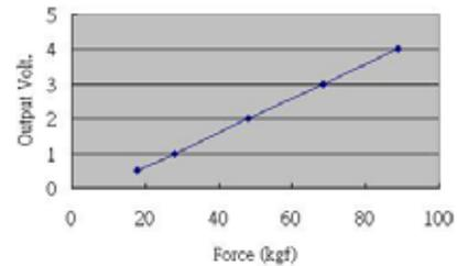
Fig. 2 The calibration of voltage-force
