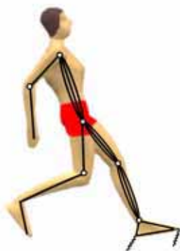
Figure 1: Eight-segment simulation model of the foot contact phase in running jumps from one leg.
