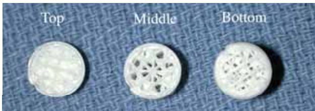
Figure 1: Scaffold showing cross layered polymer pattern. Layer labeled top is solid and has a dome shaped section above it to support tissue engineered cartilage.
