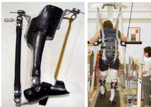
Figure 1: (a) Powered Ankle-Foot Orthosis (AFO). A lightweight carbon fiber orthosis (~1.5 kg) fit with an artificial pneumatic plantarflexor muscle. (b) Therapist Control. A therapist uses push-buttons to control the timing of active AFO assistance at the ankle as an ASIA D 24 yr. old male trains with partial body weight support.
