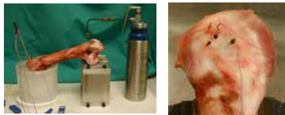
Figure 1: (a) Experimental set-up with femur in agarose and probe and thermocouples inserted into femoral head from lateral side of femur. (b) Close-up of thermocouple insertion.
