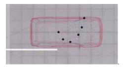
This trajectory was used to then render a 3-D drawing of occupant motion relative to vehicle interior components.
