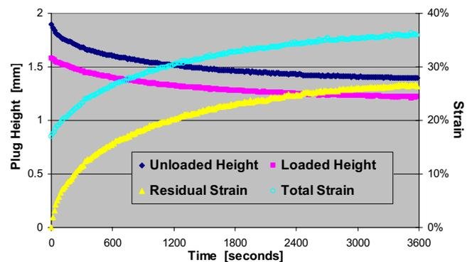
**Figure 4** Plug heights and axial strains over 1 hour of loading
