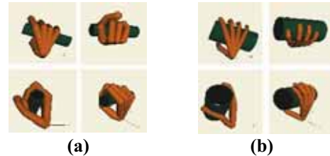
Figure 1: Predicted prehensile postures for different object and hand sizes. Left (a): a 95% male hand grasping a 20 mm diameter cylindrical object. Right (b): a 25% female grasping a 40 mm diameter cylindrical object.
