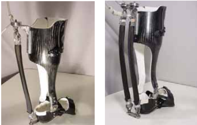
Figure 1: Powered Ankle-Foot Orthosis. Left) Orthosis fit with a single artificial muscle. Right) Orthosis fit with two parallel artificial muscles to provide plantar flexor torque.
