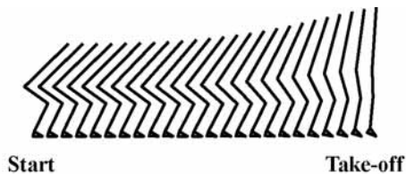
Figure 2: Stick figures of the vertical jumping of Model-Bal generated through the numerical optimization.
