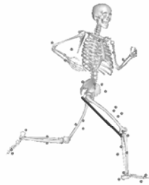
Figure 1: Musculoskeletal model shown with markers and in posture of peak hamstring muscle stretch
