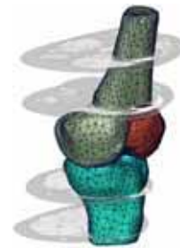
Figure 2 – Surface meshes of femur, tibia and patella developed from CT
