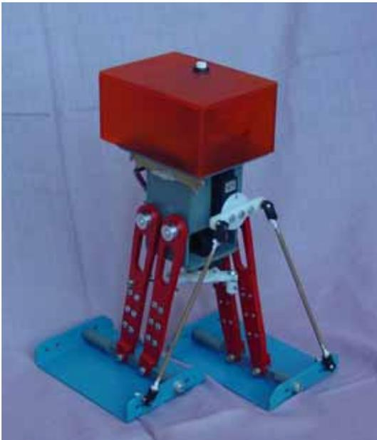
Figure 1: Powered bipedal robot driven by two motors.
