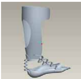
Fig. 1 Virtual ProEngineer Model of Ankle-Foot Orthoses
