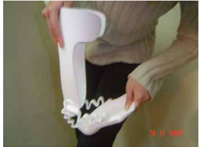
Fig. 2 Physical Model of Ankle-Foot Orthoses using Rapid Prototyping
